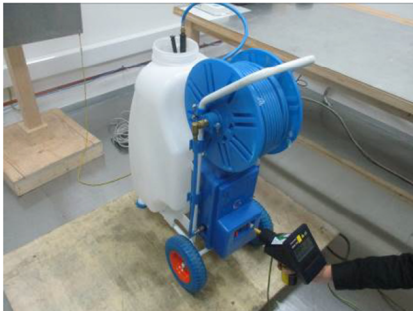
Photograph 2: Set-up for immunity test of ESD
